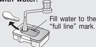
**How to remove the tank plug.**
