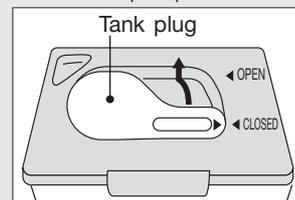
**2** Put the tank plug on the water supply tank, carry carefully without tilting it, and return to its original position.
