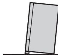
※ After several days from installing, it may sink to the floor by weight. Please re-adjust the adjustable legs again.
